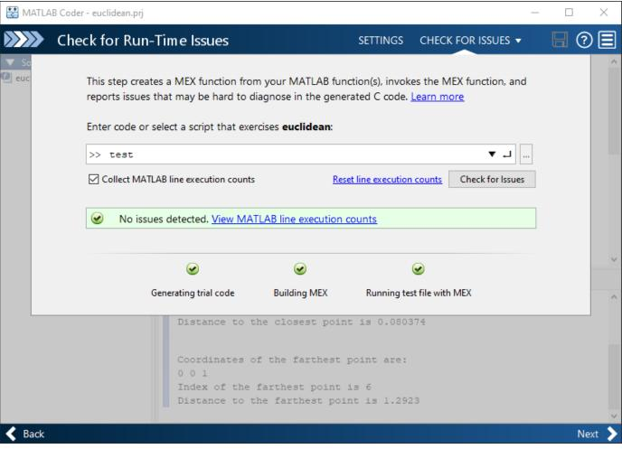
By default, the app collects line execution counts. These counts help you to see how well the test file test.m exercised the euclidean function. To view line execution counts, click View MATLAB line execution counts. The app editor displays a color-coded bar to the left of the code. To extend the color highlighting over the code and to see line execution counts, place your cursor over the bar.
