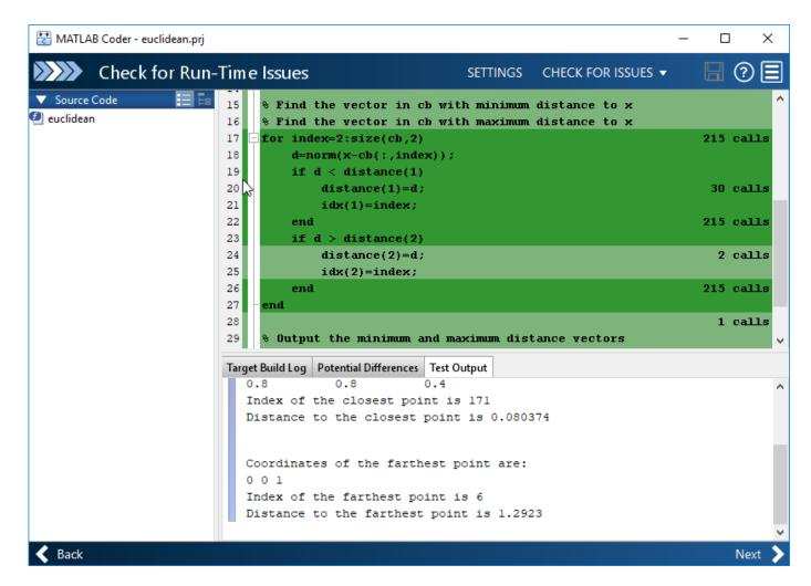
A particular shade of green indicates that the line execution count for this code falls in a certain range. In this case, the for-loop executes 215 times. For information about how to interpret line execution counts and turn off collection of the counts, see "Collect and View Line Execution Counts for Your MATLAB Code".
